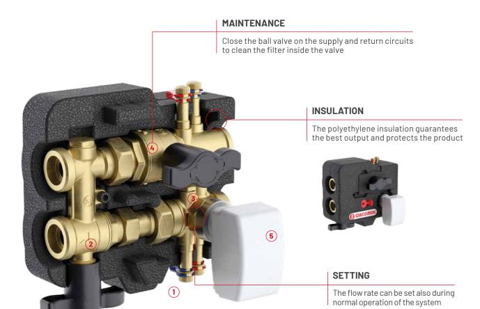
The **R280KC** pre-assembled kit consists of a diverting ball valve to bypass the unit, a full-port ball valve with integrated filter, a pressure independent control valve (PICV), a drain cock and four pressure ports to measure the differential pressure and the flow rate.
